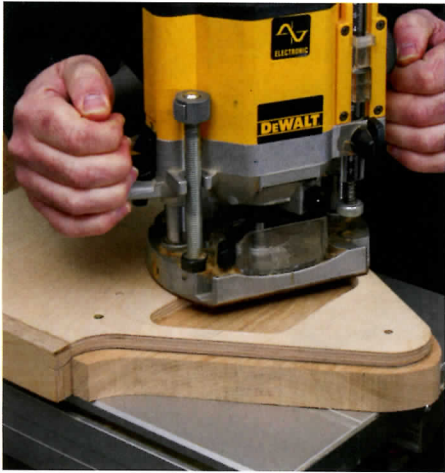
10 The main bracket web is formed using the bowl cutter
