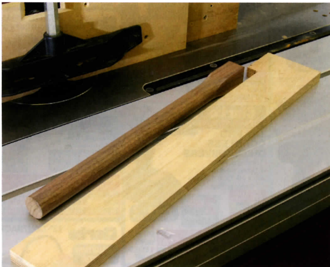
20 30mm pin blank after four passes through a half-round cutter. Shop-made push stick keeps fingers intact
