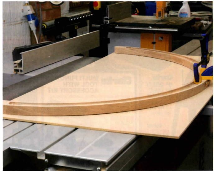
19 Two halves of the rear brace located with dowels to the assembly template and glued together with a loose tenon
