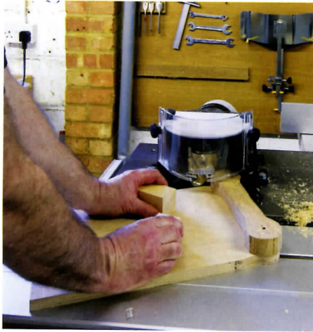
1 The first step is profiling the link form using a spiral cutter and ring guide
