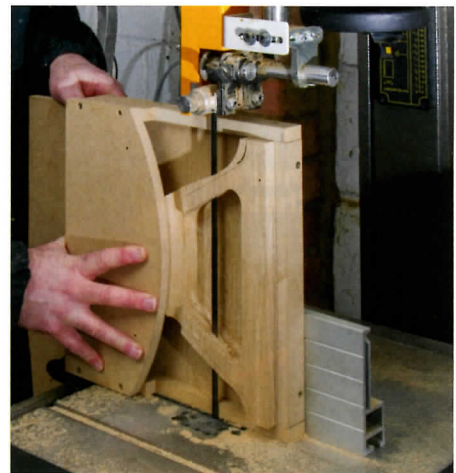
12 The bulk of the waste material of the bracket is removed on the bandsaw
