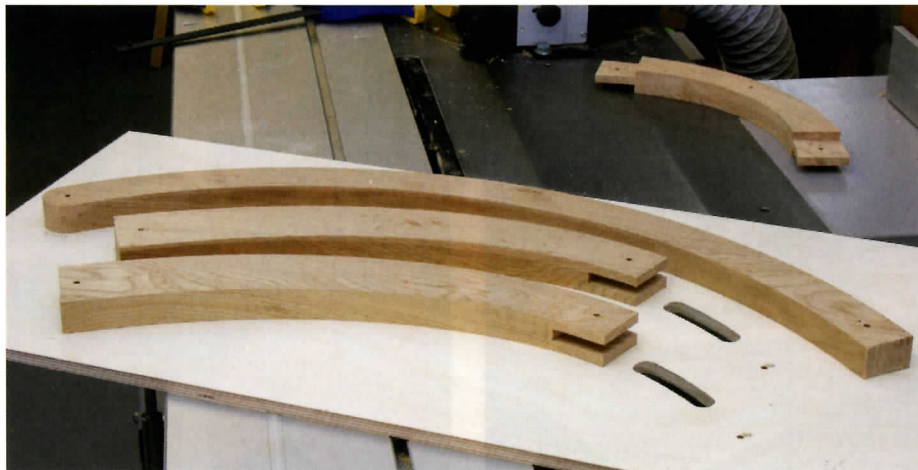
16 Two lower leg and one brace component located on the fluting template
