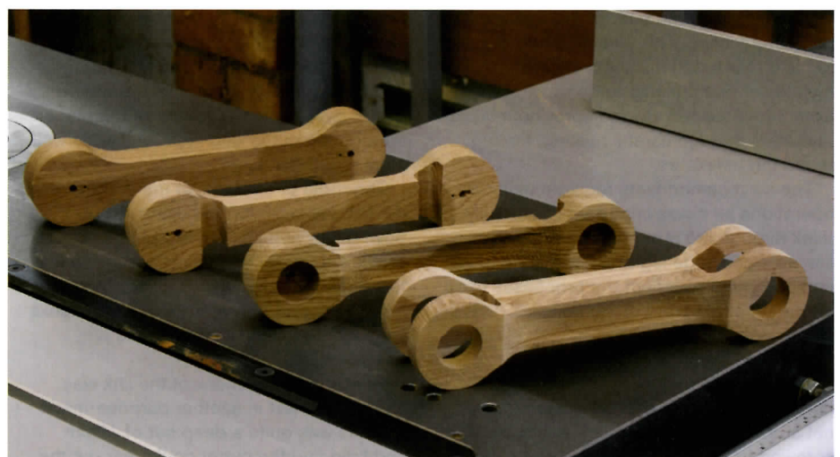
9 Progression of link operations can be clearly seen here
