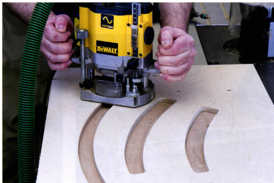
17 Machining the flutes with the bowl cutter
