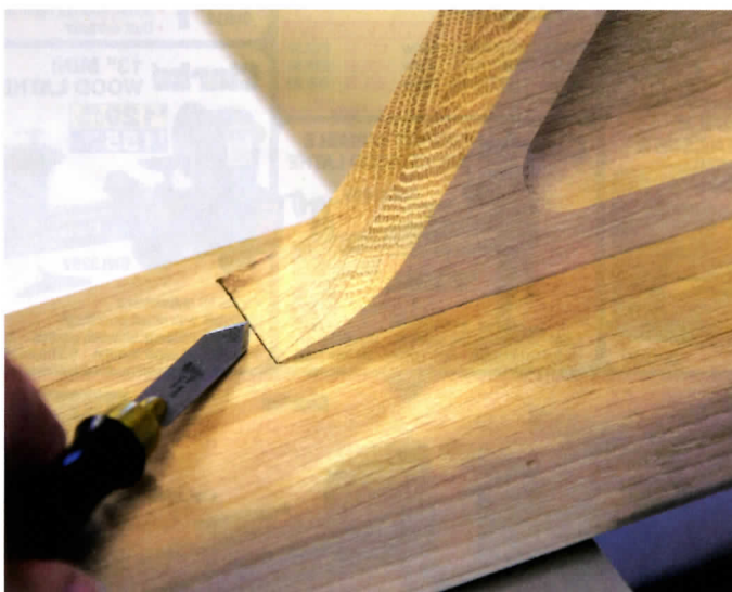
22 Leg components dry assembled and brackets scribed where necessary for adjustment
