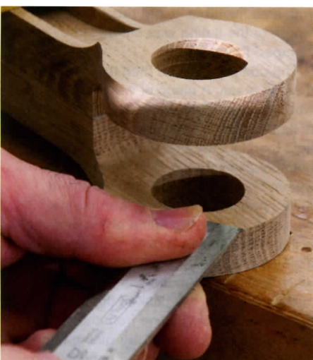
8 Final sizing of the fork is carried out by hand paring to ensure a good fit
