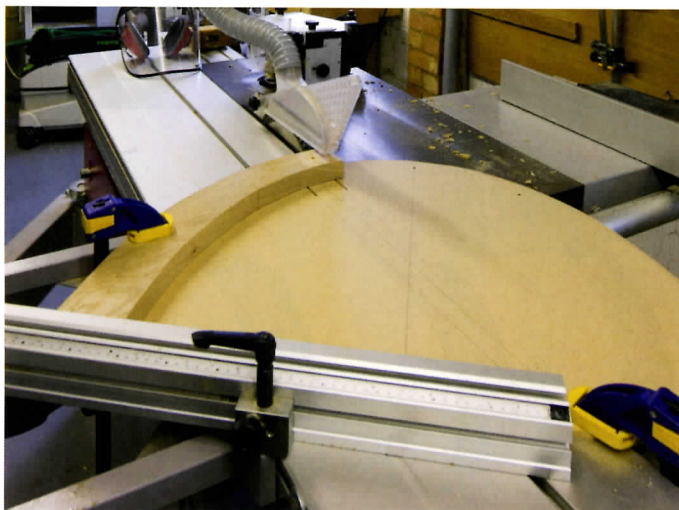
14 Precise parting of the joint end of lower leg using the full-size template
