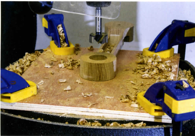
5 A gauge pin in the ply base ensures the pin hole is concentric to the profile
