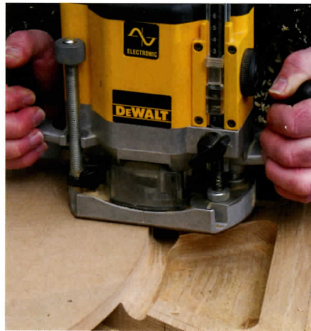
11 Transition from the boss to the upper part of the bracket is formed with a 12.5mm cutter
