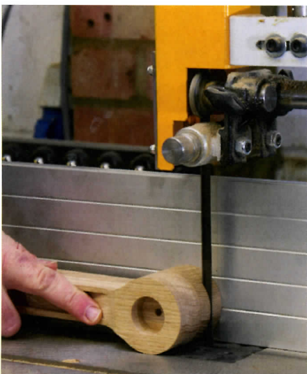
7 Waste material of the fork is removed on the bandsaw
