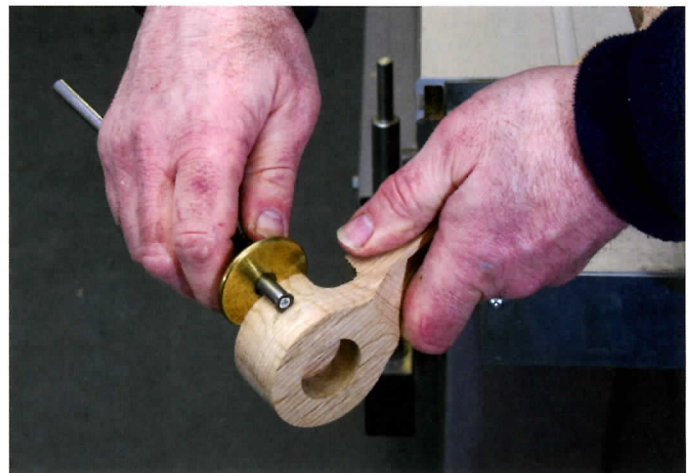
6 Scribing from the root of the fork defines the fork flank
